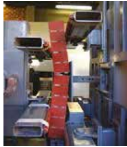
Masonry flexural strength testing in laboratory
