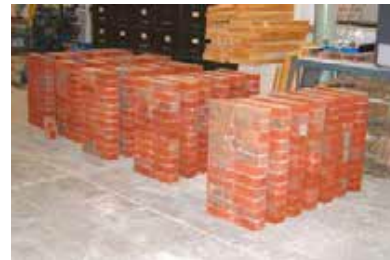
Walette sample panels for flexural strength testing.
