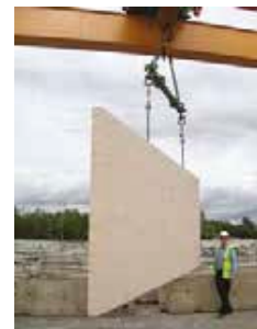
Walette sample panels for flexural strength testing.
