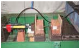
Testing of wall ties for prefabricated cavity wall manufacture
